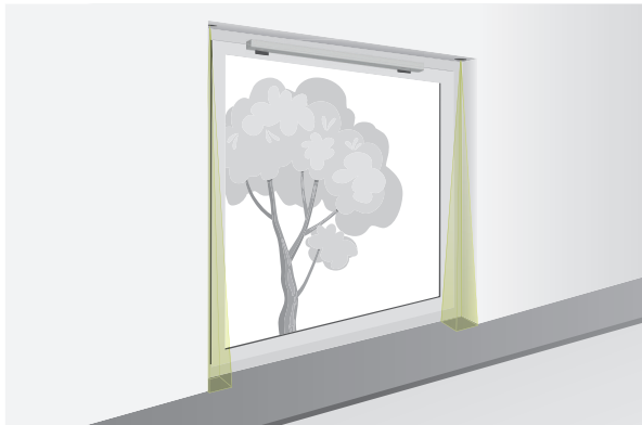
Fig. 4: Closing edge safety device on automatic windows
